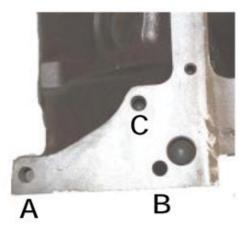
Convert Chevrolet 6 cylinder and Small Block V8 with 2 bolt hole started pad to a universal 3 bolt hole.
